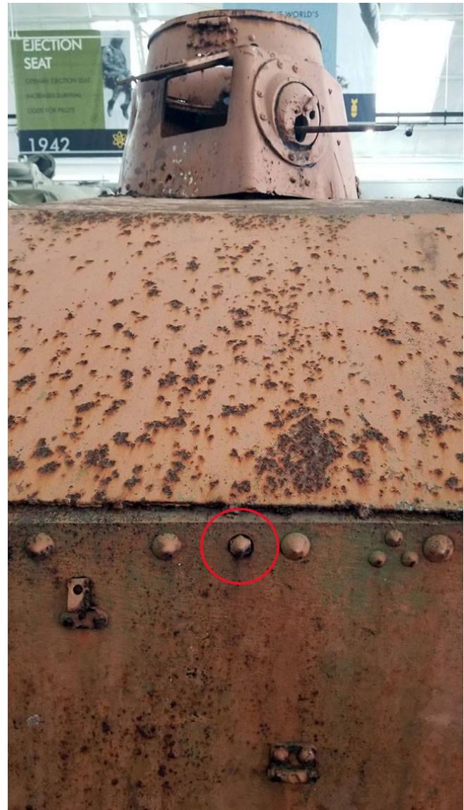
One of these is not like the others. A Type 95 Japanese tank featured a dummy rivet (circled in red) that actually was a button for infantry to notify the tank's crew of their presence. (Flying Heritage Combat Armor Museum image)
